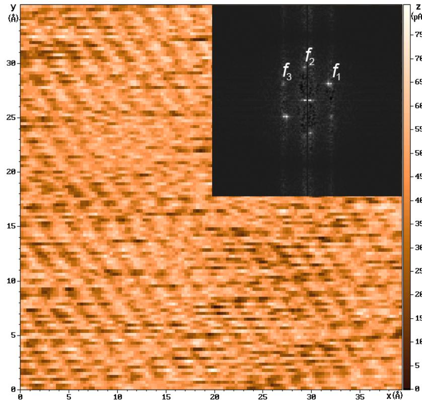
STM scan after Fourier filtering
