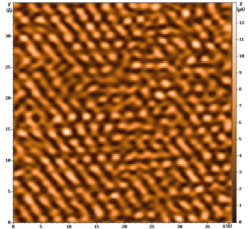
Lattice constants:  $a_1=2.1 \text{ \AA}$ ,  $a_2=2.8 \text{ \AA}$ ,  $a_3=2.1 \text{ \AA}$ . Crystallographic directions:  $\theta_1=131.1^\circ$ ,  $\theta_2=4.7^\circ$ ,  $\theta_3=58.0^\circ$
