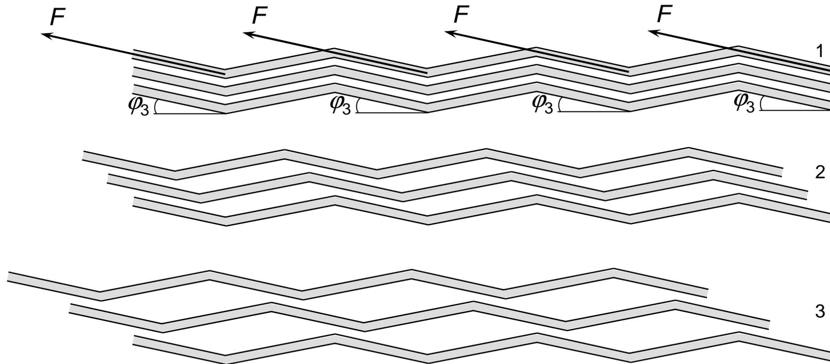
Two channel layers are composed of three split-in-folds graphene layers by means of relative shifting (sliding) of these layers along plane of a small facet
