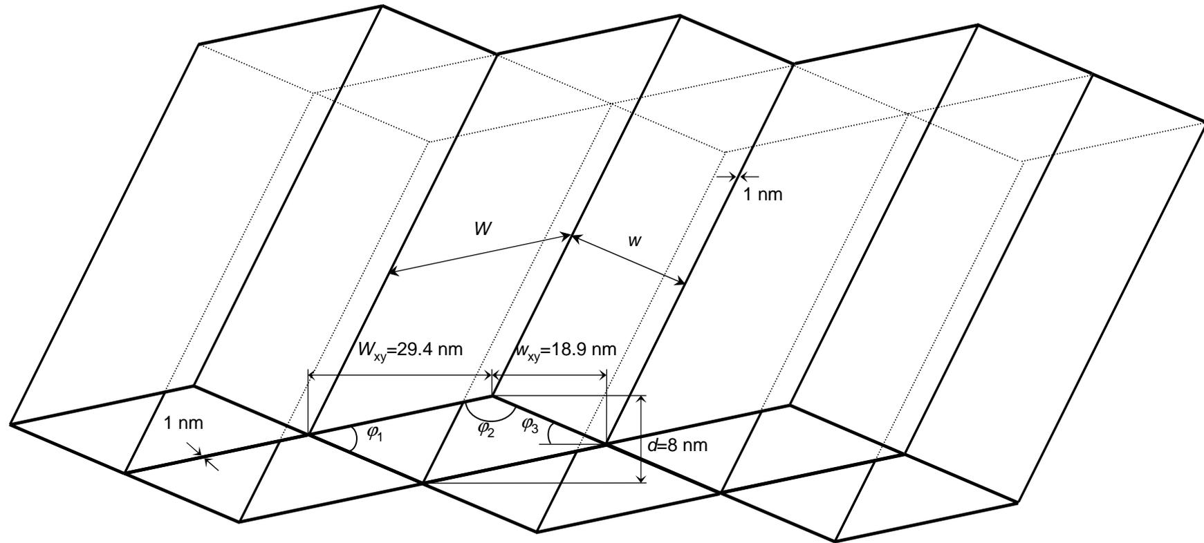
Width of small facet  $w=19.3 \text{ nm}$ , width of large facet  $W=29.7 \text{ nm}$ ,  $\varphi_1=19.7^\circ$ ,  $\varphi_2=160.3^\circ$ ,  $\varphi_3=12.0^\circ$
